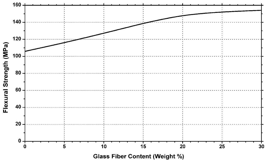
Figure 10.82. Flexural strength vs. glass fiber content of Solvay Advanced Polymers Udel® PSU resins.
